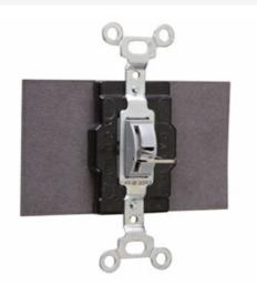
Single Pole, Double Throw Switch. 15 Amps, 120/277VAC rating, Locking. Tested to 3 Amps, 24Vdc rating.
