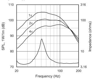
4642A frequency response and impedance (bottom curve), 1 watt at 1 meter, with 150 Hz Linkwitz-Riley 4th order low-pass filter measured under  $4\pi$  ground plane conditions.  $1\pi$  (upper curve) and  $2\pi$  (center curve) loading condition predictions also shown.
