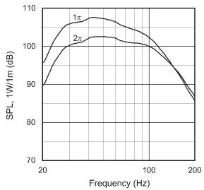
4642A frequency response, 1 watt at 1 meter, with 150 Hz Linkwitz-Riley 4th order low-pass filter and 2nd order high-pass filter at 25 Hz with Q=2.  $1\pi$  (upper curve) and  $2\pi$  (lower curve) conditions
