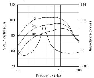
4645C frequency response and impedance (bottom curve), 1 watt at 1 meter, with 150 Hz Linkwitz-Riley 4th order low-pass filter measured under  $4\pi$  ground plane conditions.  $1\pi$  (upper curve) and  $2\pi$  (center curve) loading condition predictions also shown.
