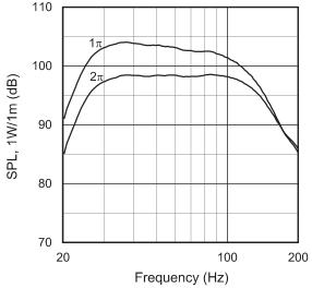
4645C frequency response, 1 watt at 1 meter, with 150 Hz Linkwitz-Riley 4th order low-pass filter and 2nd order high-pass filter at 25 Hz with Q=2.  $1\pi$  (upper curve) and  $2\pi$  (lower curve) conditions
