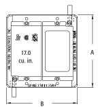
Non-metallic, combination power and low voltage box. For power, phone/cable, and fiber optic installations.
