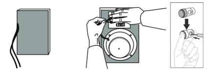
3. Place the speaker into the wall and tighten all of the dog ear screws with a Phillips screwdriver
