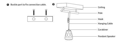
NOTE: Make sure the speaker is properly secured to the building's structure. Please use the proper screws, bolts, or anchors as failure to do so may cause the speaker to become unsecured and cause potential damages and injuries.
