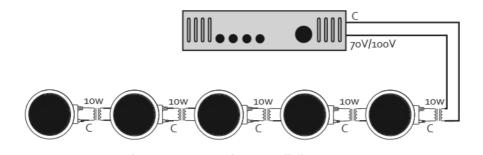
The total number of speakers multiplied by the tap value cannot exceed the output power (in watts) of the 70V/100V amplifier. The example above shows 5 total speakers. Using the 10W taps, you will need an amplifier with at least 50W (5 speakers x 10W tap).
