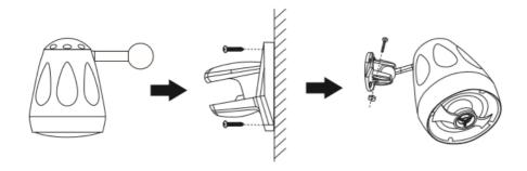
NOTE: When mounting the speaker to the wall or ceiling, make sure the proper screws and/or holts are used.
