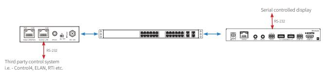
**Please note:** Only one method of RS-232 pass-through can be used at the same time. It is not possible to mix different methods of RS-232 control simultaneously.
