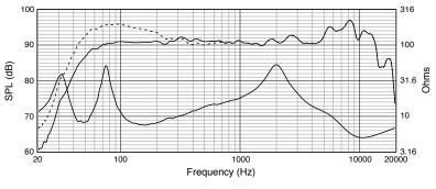
On axis in half-space (2pi, dotted line) and full-space (4pi, solid line) at thru (8 ohm) setting Input Impedance
