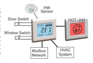
Regardless of the need to control conferential HVAC systems, 2 or 4 pipe fan coils with modulating valves the SMT-131 has the necessary outputs to achieve your control needs.
