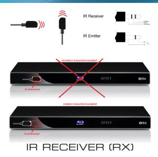
To control the source: Plug IR Receiver into IR RX port of receiver unit (EVEXHDARC-RX); place receiver at or near display.
