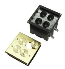
Tamper-Resistant Floor Box Assembly, Two #8 duplex openings, Four threaded screw plugs. Includes two 3232 15 amp, 125 volt tamper-resistant duplex receptacles. Brass. For detailed Tamper-Resistant receptacle information, visit our Tamper-Resistant Receptacles page.
