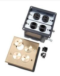
Tamper-Resistant Floor Box Assembly, Dual-voltage. Two #8 duplex openings, Four threaded screw plugs. Includes 3232 15 amp, 125 volt tamper-resistant duplex receptacle, Cat5E Jack, F-connector, Ten Blanks and a low-voltage divider. Brass. For detailed Tamper-Resistant receptacle information, visit our Tamper-Resistant Receptacles page.
