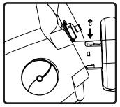
8. If speaker is within reach of the public, or extra security is desired, install the included M3x4mm security screw.
