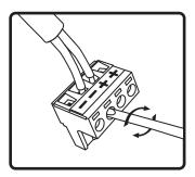
4. Connect signal wire to 4-pin Euroblock plug. Tighten unused terminal screws. Use inside positive and negative inputs for either voice coil or distributed systems. For daisy chaining, use outside positive and negative terminals.
