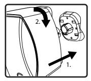
7. Line up bracket ribs with mounting tube slots and press speaker onto bracket. Twist clockwise until speaker clicks. Speaker is now locked in place.
