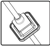
3. Slip terminal weather boot over signal wire. For environmental applications, put RTV silicone around nipple and base when installation is complete.
