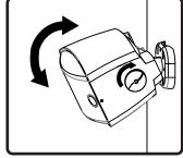
10. Make sure knob is loose, and aim speaker in desired direction (0 to 90). Tighten the knob to lock the speaker in place. FINGER TIGHT IS SUFFICIENT- DO NOT OVER TIGHTEN.
