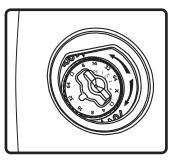
11. Select the tap position by removing the rubber plug on grille to access rotary switch. Switch is preset to maximum tap setting in 70.7V mode. Select desired setting and reinsert rubber plug.
