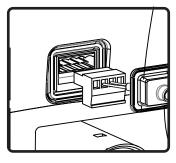
5. Insert 4-pin Euroblock plug into Euroblock jack on rear of speaker. Connectors are keyed for polarity. Terminal weather boot will seal the enclosure on rear of speaker.
