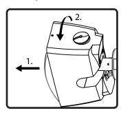
9. Firmly grip speaker and pull it away from the wall to rotate to to desired mounting angle about the mounting shaft axis. Simply release speaker back toward the wall to lock into place.
