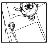
6. Use supplied screw to connect the safety cable to one of the inserts on the rear panel of the speaker. Connect other end of the safety cable to a secure mounting point.
