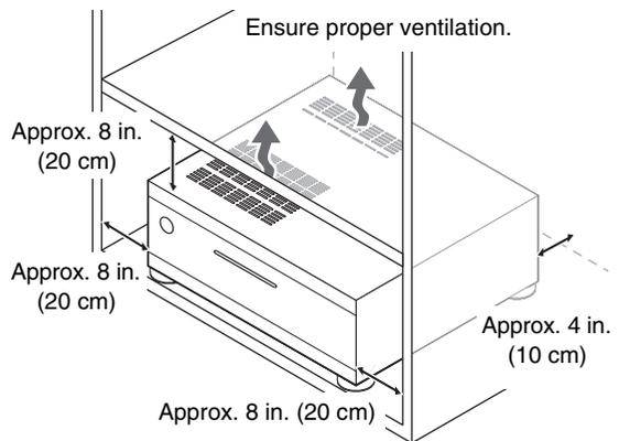
Install the power amplifier on a sturdy rack or shelf. Position it so that its weight is evenly dispersed on its four legs. Do not install the power amplifier in a place with vibration or an unstable location.
