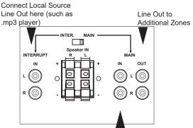
Use these Inputs to connect Pre-amp or Receiver Line Out
