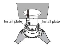
(2) Rotate the product inwards to fit properly onto the surface of the drywall. Once inside the hole, release the install plates.
