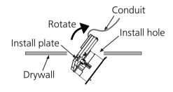
(3) The install plates will position themselves onto the drywall.
