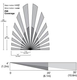
For best performance, WattStopper recommends using this sensor in spaces no larger than  $15^{\circ}$  x  $12^{\circ}$ .
