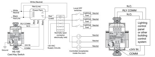
Do not wire receptacles directly to HS-100; device is not rated to control receptacles
