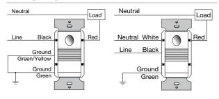
Wiring for PW-100 with no neutral wire run to the switch box.
