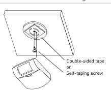
Sensor mounts under desk or binder bin with double-sided tape or self-taping screw
