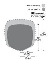
For best performance, WattStopper recommends using this sensor in spaces no larger than 15'  $\times$  15'.
