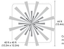
Multi-level, 360° Fresnel lens for superior occupancy detection
