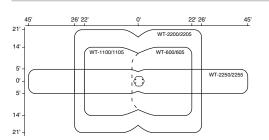
Coverages shown represent half-step walking motion. Actual coverages can vary for each application depending on the shape and use of space and the obstacles present. Coverage may be reduced if product is mounted greater than 12 feet high.
