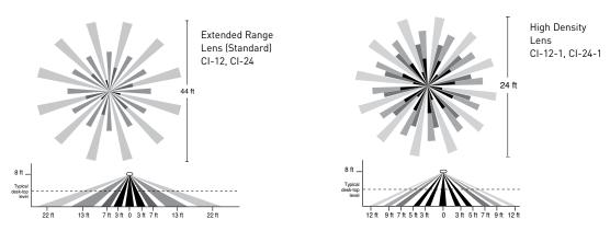
Coverage shown is maximum and represents coverage for half-step walking motion. Under ideal conditions, with no barriers or obstacles, coverage for half-step walking motion can reach up to 1200 ft² using the Extended Range lens and up to 500 ft² using the High Density lens. For typical desktop level of activity, coverage can reach up to 300 ft² using the High Density lens.
