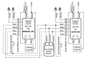
By using two low-voltage switches, a ceiling sensor and two BZ-150s (one set to Auto ON and one set to Manual ON) bi-level switching with manual-on operation can be achieved.
