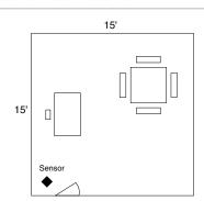
For an enclosed office, the WPIR should be placed in the corner of the room so that it will detect occupants as they enter the room. For the aisleway between bookstacks, the WPIR should be placed at the end of each bookstack to detect occupancy upon entrance to the aisle way from either direction. For longer bookstacks, two or more WPIRs can be used.
