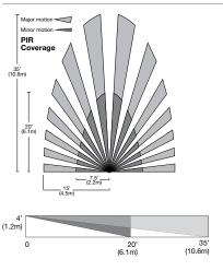
For best performance, WattStopper recommends using this sensor in spaces no larger than 15' x 12'.
