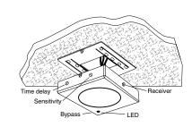
Attach sensor to a vibration-free surface. Mount the sensors with the receivers facing the area of coverage. Note: Ultrasonic sensors should be placed 4' away from supply ducts, 6' from horizontal discharge ducts, and 6" from power packs.
