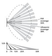
Coverages shown are maximum and represent half-step walking motion. Under ideal conditions with no barriers or obstacles, coverage for half-step walking motion can reach up to 2000 ft², while coverage for typical desktop activity can reach up to 1000 ft2.
