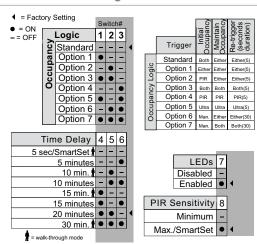
The technology control (occupancy logic) options are adjustable by user. The standard setting (recommended for most applications) is both technologies to trigger on, either to hold on.
