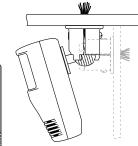
A swivel mounting bracket attached to the sensor allows the sensor to be angled for wall or ceiling mounting.
