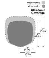
For best performance, WattStopper recommends using this sensor in spaces no larger than 15'  $\times$  15'.
