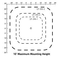
Coverages shown represent half-step walking motion when sensor is mounted 8'-10' high. Actual coverage can vary for each application depending on the shape and use of space and the obstacles present.
