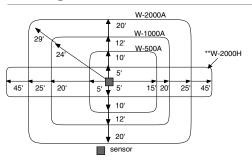
Coverage shown represent half-step walking motion. Actual coverage can vary for each application depending on the shape and the use of space and the obstacles present. Coverage may be reduced if product is mounted greater than 12 feet high.
