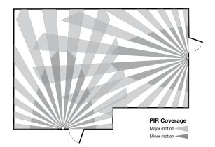
For best performance in single location applications, WattStopper recommends using this sensor in spaces no larger than 15' x 12'. In multi-way applications, each connected sensor expands the coverage area.
