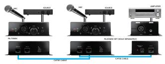
To add additional sources, the PA-EXMIX allows for cascading additional PA-TXMIX Transmitters (sold separately). See below for connecting an additional Transmitter:
