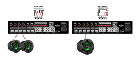
The PA66MK2 can work with speakers that are 4-8 Ohm. There are two modes that can be set for different setups: Stereo or Bridge. An 8 Ohm speaker can only be used when in Bridge mode. To choose between modes, use the mode switch to determine modes for each zone (Number 2 Panel Descriptions, page 5)
