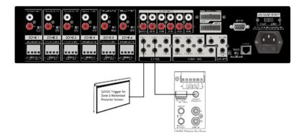
There are six 12VDC trigger outputs which correspond to the six output zones. When a zone is powered ON by the PA66ACCS keypad, the corresponding zone sends 12Vdc to the trigger output jack. The triggers can be used to automatically switch peripheral equipment ON or OFF.
