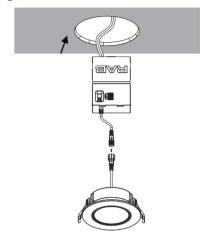
7. Lifting both retention tabs upward. Push until the trim sits flush against the ceiling. (Fig.6)
