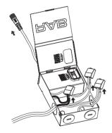
5. Place all wiring and connections back into the box, close the cover and select desired CCT. (Fig.4)
