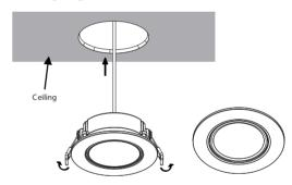
8. Push the edge of the bezel to tilt lens. Rotate lens assembly horizontally towards the surface to be illuminated. (Fig. 7)
