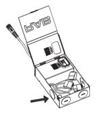
4. Insert the electrical supply cable through the knockout and secure with a terminal. Wire driver box (*Fig.3*), white-white, black - black, green - green/ground.
