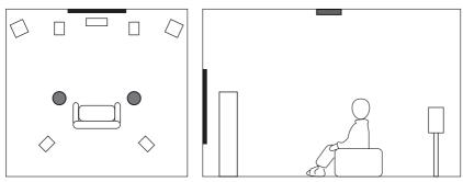
• When installing 4 presence speakers to a ceiling, install 2 front presence speakers to the ceiling between the extensions of the front speakers and listening position, and install 2 rear presence speakers to the ceiling between the extensions of the listening position and surround (or surround back) speakers.
