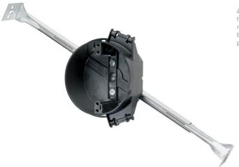
4" Round Ceiling Box with abar hanger that adjusts to 16" or 24" joist spacing. It has four Auto/Clamps. It is constructed with impact-resisitant Noryl thermoplastic, making it virtually unbreakable and non-conductive. Its depth-mounting gauge at bottom of bracket helps you align the box at the proper depth relative to the ceiling. 50 pack.
