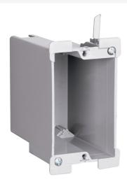
Single gang, deep old work switch and outlet box with Quick/Click and Swing-Bracket for mounting, adjusts from 1 1/4" down to 1/8". It has twoAuto/Clamps foreach end. It has a durable, impact-resistant thermoplastic box. The metal swing bracket is for quick mounting in existing walls. 50 pack.
