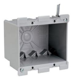
Double Gang, Old Work Switch and Outlet box with swing-bracket for mounting, adjusts from 1 1/4" to 1/8". It has four Auto/Clamps for each end. It has a durable, impact-resistant thermoplastic box. The metal swing bracket is for quick mounting in existing walls. 50 pack.
