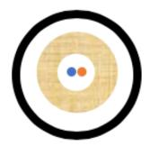
*S2I-2M-P-BK* fiber optic cable is constructed with two internal tight buffers, internal aramid yarn, and one outer plenum-rated PVC jacket in distribution format. The fiber cable features a water-resistant jacket and is designed for indoor and outdoor applications.
