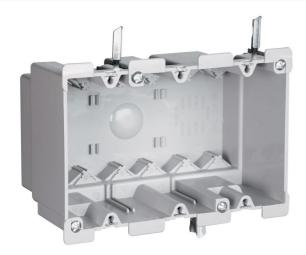
Triple Gang, Old Work Switch and Outlet Box with Swing-Bracket for mounting. Adjusts from 1 1/4" down to 1/8". Six Auto/Clamps for Each End. 10 pack.
