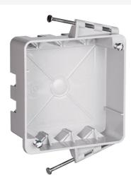
$4" Square Box with threaded mounting holes, captive mounting nails each end. 3 \\ Auto/Clamps each end, 2 on side opposite to nails. Two #8Mounting Screws Factory Installed.$
