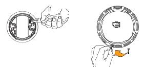
3. Push the locking pin through the hole near the battery drawer on the back of the Alarm.
