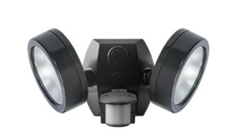
Two adjustable 13W LED floodlights. Equivalent to 2x75W BR30/halogen/wide floods. Comes with sensor with 180° detection pattern at up to 30 ft. Weight: 5.5 lbs
