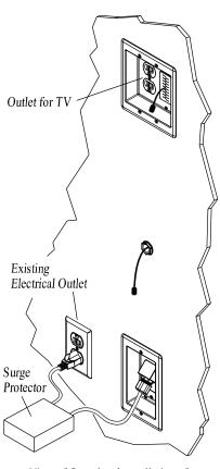
View of Completed Installation of TVBRA3K Pre-Wired TV Bridge
