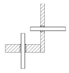
Install sealant to required depth. Work sealant into all areas exercising care to eliminate voids or seams. The surface of the sealant can be smoothed using a putty knife dipped in water. Adding water to the sealant itself is not recommended.
