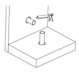
Sealant may be installed by caulking using a standard caulking gun or from bulk containers using a bulk loading caulk gun, or by manually troweling using a mason's trowel or putty knife.
