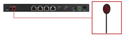
2. Plug the IR Receiver into the IR IN Port of the receiver unit; place receiver at or near display
