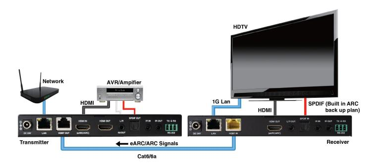
The Evolution by Vanco EVEXHDB3 HDBaseT 3.0 extender offers multiple options for pass-through control, and audio including eARC and ARC, along with PoH while being able to extend uncompressed 4K with HDR up to 164ft/50m over a single Cat6 or up to 328ft/100m using Cat6a/7.
