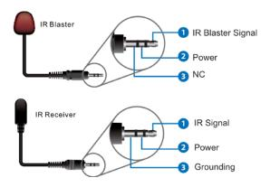
NOTE: Infrared receiving areas of source devices can be located by shining a flashlight onto the front of the device – the sensor should be able to be seen through the plastic as a small, round object inside. Place the IR Emitters around or near this area with the tip of the IR emitter near the IR sensor of the source. IR receivers should be placed at the display and line of sight, so that an IR remote can be pointed at the pigtail to receive IR signals.
