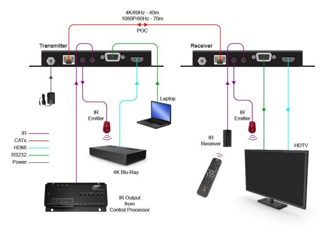
Plug the IR receiver into the ZIG-POC-70L-Tx "IR IN" port and place the IR receiver so you can point to it easily with your IR remote controller.
