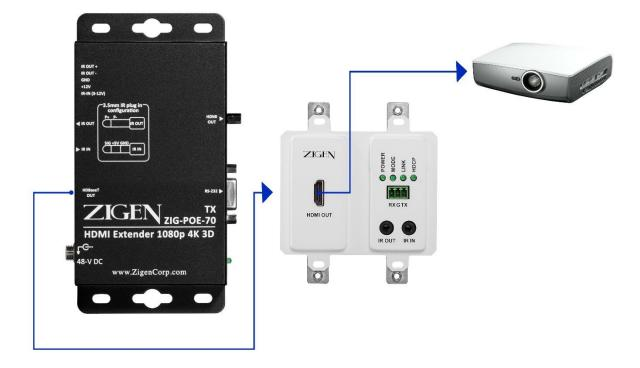
Example is showing our HDBaseT Transmitter ZIG-POE-70 connected to the ZIG-POEWP-Rx70 HDBaseT receiver wall Plate with IR and RS232 control.
