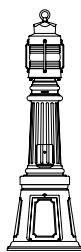
B8646 H: 41 3/4" W: 13 1/8" Anchor base with 7" dia. bolt circle. (four bolts supplied)
